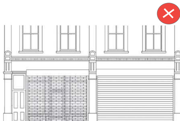
Picture 66. External Roller shutters are not appropriate.
